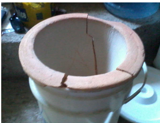
Figure 8: (clockwise from top left) DR Atabey Ceramic Filter, a Haiti FilterPure Ceramic Filter, a Broken Ceramic Filter, a DR Atabey Filter Unit
